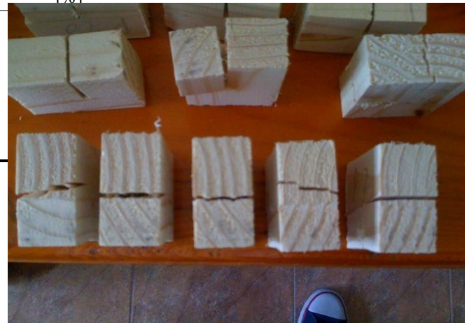
Figure 5. Wood failure of fir's test pieces
