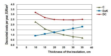
Figure 3. Dependence between the thickness of the reed roof and the relative costs in using "Donbaski" coal for fuel.
