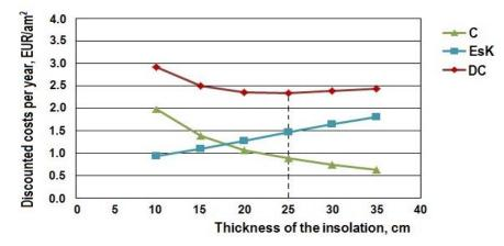
Figure 2. Dependence between the thickness of the reed roof and the relative costs in using pellets for fuel.
