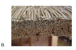
**Figure 1.** Reed bladed slabs from longitudinally located sheaves (stems thickness 0.2 - 0.5 cm).
