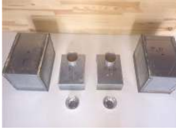
Figure 2. Devices for kinetic analysis of adsorption. On each side, are presented the equilibrium cases; down; the empty nacelles; in the middle, the filled nacelles on their supports.
