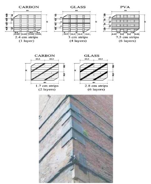
Figure 6. Single-side or double-side strengthening with FRP strips or steel ties
