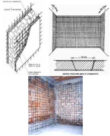
Figure 8. R.C. jacketing reinforcing
