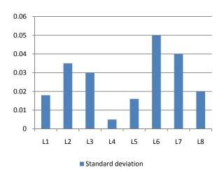
**Figure 2.** Graphic presentation of standard deviation of total solids determination for 8 labs.
