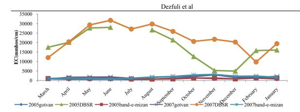
Figure 4: Monthly changes of salinity (electrical conductivity) in 2005 and 2007 water separation stations (µmohs /cm)
