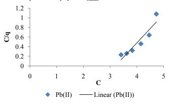
Figure 6.Langmuir isotherm plot for Pb (II)
