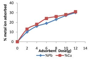
Figure 2.Effect of adsorbent dose on adsorption
