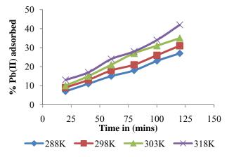
Figure 4 : Effect of temperature on Pb (II)
