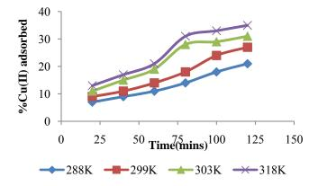
Figure 5 : Effect of temperature on Cu (II)
