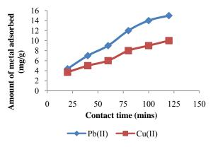
Figure 3: Effect of contact time on adsorption
