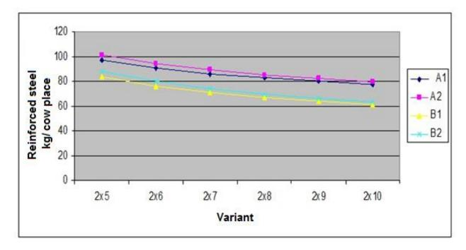
Figure 1. Effect of milking parlour capacity on the relative weight of reinforced steel per cow place in a conventional exit variant
