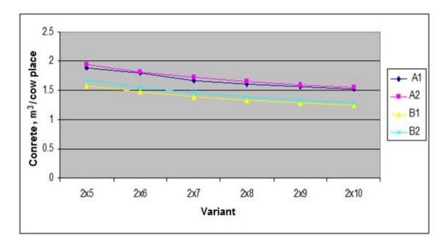
Figure 4. Effect of milking parlour capacity on the relative amount of concrete per cow place in a conventional exit variant
