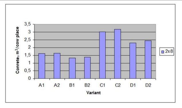
Figure 5. Comparative analysis of the relative amount of concrete for herringbone parlours with different positioning angle and different entry/exit variant
