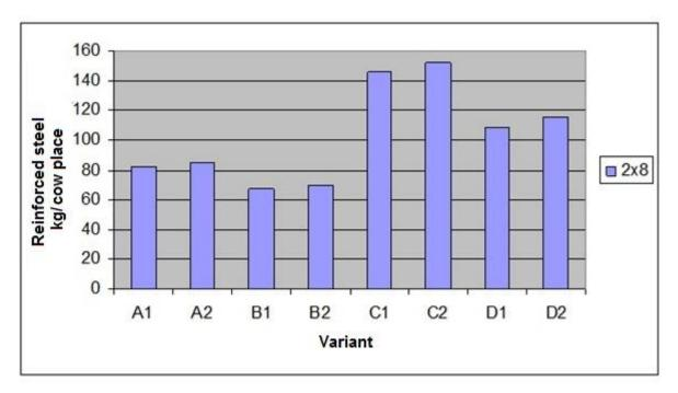
Figure 2. Comparative analysis of the relative weight of reinforced steel for herringbone parlours with different positioning angle and different entry/exit combination
