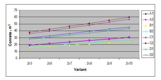
Figure 3. Absolute amount of concrete spent for herringbone parlours with different positioning angle and different entry/exit variant
