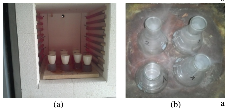
Figure 1. Samples treatment: a) combustion in a furnace), b) treatment with nitric acid
